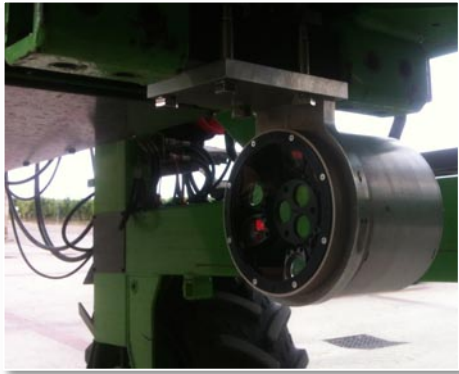
Mounted Multiplex for hot-spot detection
