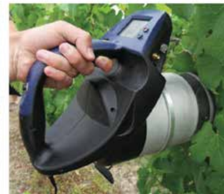
Deposits quantification on leaves with the MULTIPLEX® sensor
